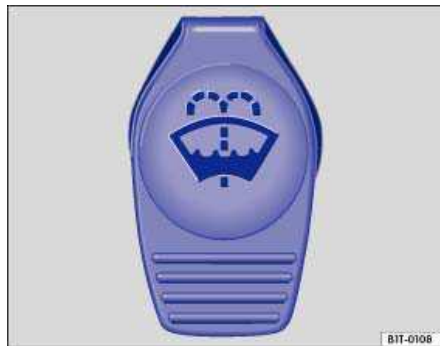
Fig. 84 In the electric motor compartment: Cap of the windshield washer fluid reservoir.
