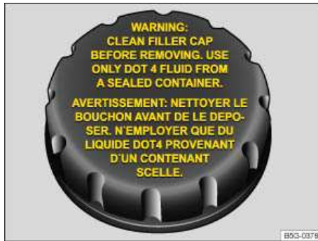
Fig. 130 In the electric motor compartment: Brake fluid reservoir cap (cap design may vary depending on vehicle equipment).
