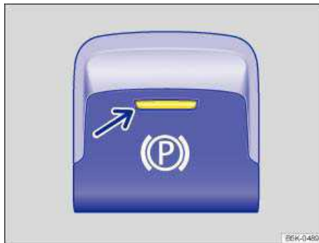
Fig. 129 In the lower section of the center console: Electronic parking brake button.
