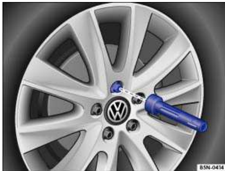
Fig. 176 Changing a wheel: Remove previously loosened wheel bolts using the screwdriver handle.
