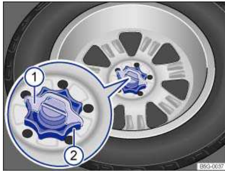
Fig. 101 In the luggage compartment: Handwheel holding the spare wheel in place (if equipped).
