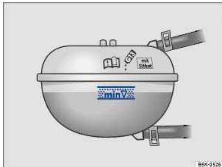
Fig. 154 Coolant expansion tank in the electric motor compartment.
