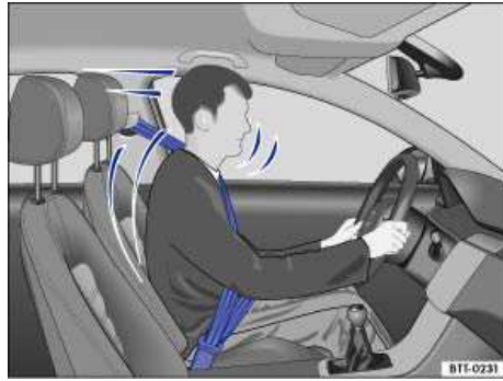
Fig. 51 Belted driver secured by the correctly worn safety belt in the event of a sudden braking maneuver.
