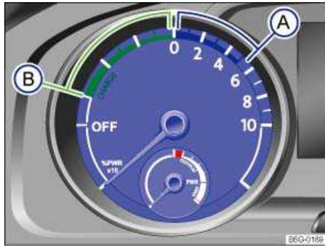
Fig. 123 In instrument cluster: power display with ranges for energy consumption A and for recuperation B
