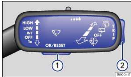
Fig. 13 On the right side of the steering column: Windshield wiper lever with controls for instrument cluster menus and displays.
