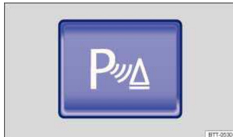
Fig. 146 In the center console: Button to switch the Park Distance Control system on or off.
