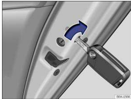
Fig. 162 On the front side of the right rear door: Locking the vehicle with the key bit in the vehicle key.
