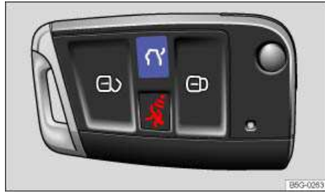
Fig. 27 In the remote control vehicle key: Button to unlock the rear hatch.
