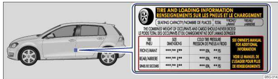
Fig. 99 On the driver door jamb: Location of the tire inflation pressure label.
