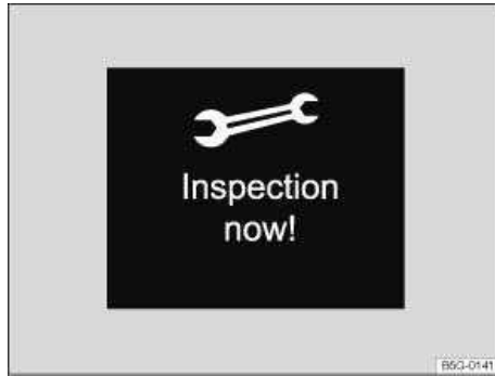
Fig. 11 In the instrument cluster display: Example of the service reminder when a service is due.
